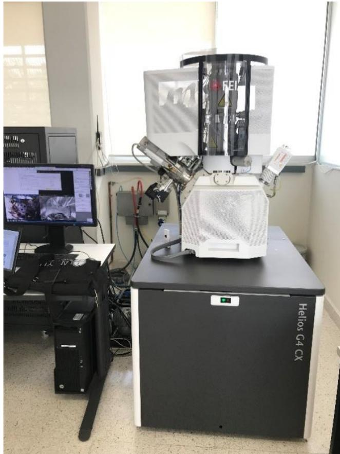
**Figura 3.8.** Microscopio Dual Beam Helios G4 CX.
